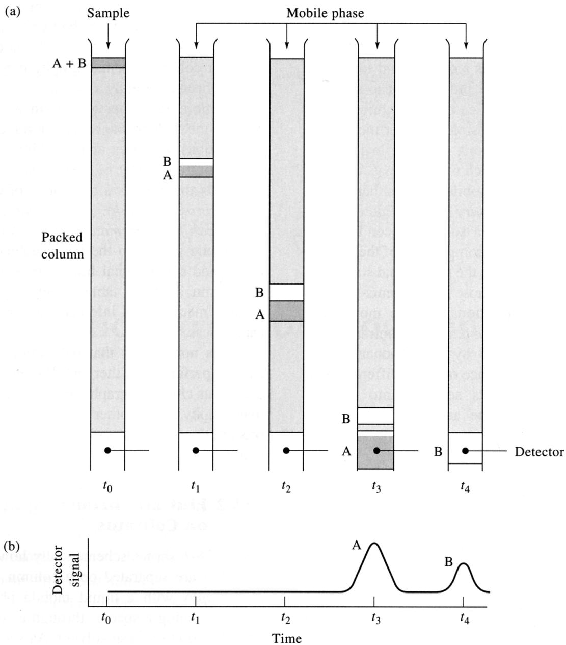
**Figure 26-1** (a) Diagram showing the separation of a mixture of components A and B by column elution chromatography. (b) The output of the signal detector at the various stages of elution shown in (a).
